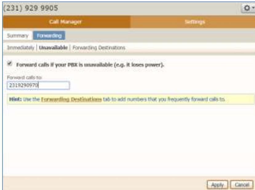
12. Click the **Apply** button to save the change. Calls to this telephone number should now ring to the destination number if the SIP PBX is unavailable.
